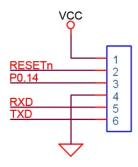
The ISP function uses only six pins: VCC, GND, RXD, TXD, P0.14 and RESETn. The simple circuit above is all that must be added to the user's application to use ISP with USB-ICP.
